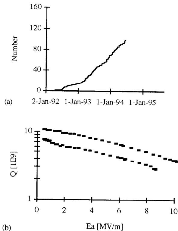
Fig. 1. a) Total number of accepted cavities (vertical test) vs. time for the series production of 168 NbCu cavities. b) Q-value at 4.2 K vs. accelerating gradient for two cavities from one company with the best and (contractually tolerated) worst performance. Cavities from the other companies behave similarly. The lower curve has originally been measured at 4.5 K, but for comparison, the data were extrapolated to 4.2 K.
