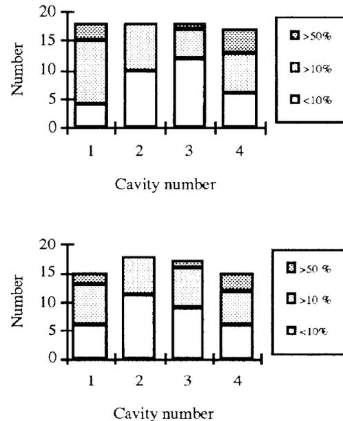
Fig. 4: Histogramm of number of cavities having undergone a degradation after assembly. The relative change (in %) of RF loss between the vertical test and the horizontal test is shown. The upper plot refers to the RF loss at low field, the lower plot to the RF loss at 6 MV/m. Numbers below 10% are insignificant. Cavity numbers 1 and 4 are located at the end of the cryo-modules, 2 and 3 are located in the middle. The degradation is larger in the end cavities.
