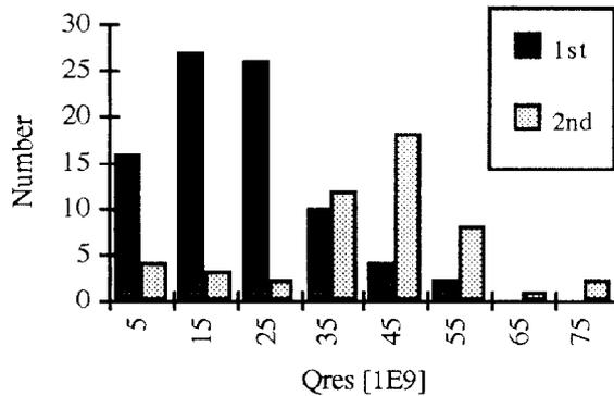
Fig. 3: Residual Q-value for first and second coating.
