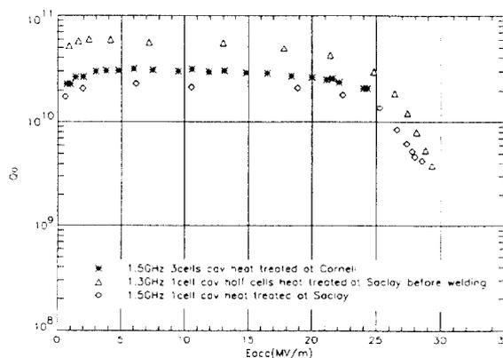
Figure 1 Q value vs accelerating gradient for three heat treated "high gradient" cavities
