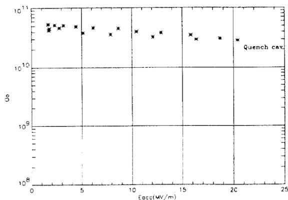
Figure 2 Q value vs accelerating gradient for a "low dissipation" cavity
