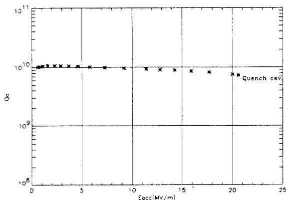
Figure 4 Q value vs accelerating gradient for a cavity equipped with a demountable HOM coupler
