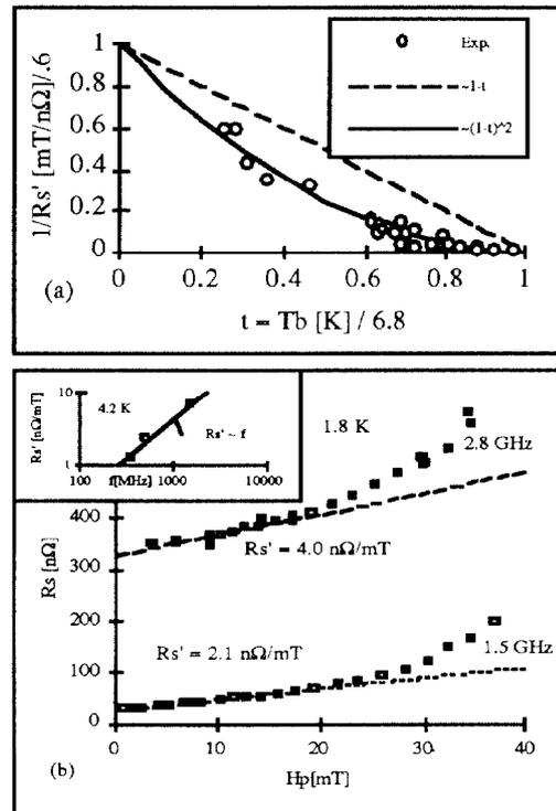
Fig. 4: Non quadratic loss (NQL) measured vs. the bath temperature  $T_b$  (a) and vs. the RF magnetic peak field amplitude  $H_p$  at 1.5 GHz and 2.8 GHz in the same cavity (b). The inset is explained in the text.
