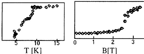
Fig. 2: Secondary coil voltage (arb. units) for measuring the critical temperature  $T_c$  (left) and the upper critical field  $B_{c2}$  (right) on a niobium layer sputter coated on a copper substrate. The RRR was 12 for this particular sample, and the temperature during coating was not controlled.
