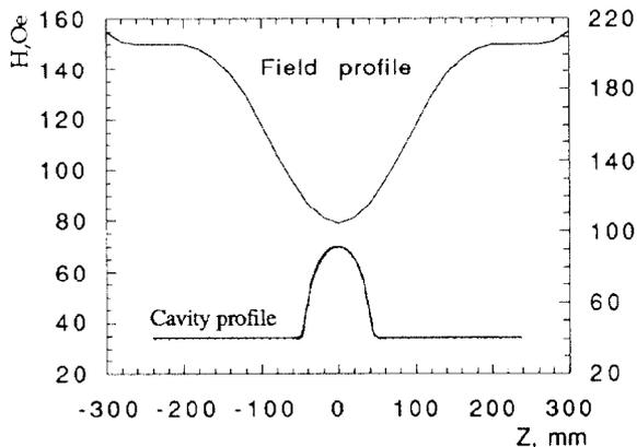
Fig. 1 Parallel component of the magnetic field profile along the cavity axis for the post-magnetron we built.
