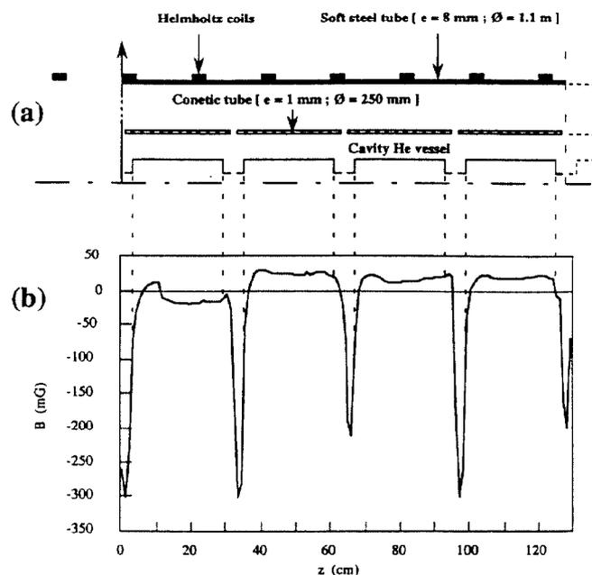
Figure 1. a) A mixed scheme for TESLA TTF cryomodule, b) Field profile measured along the z-axis on a scale 1/4 model
