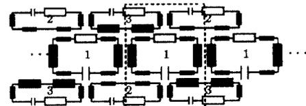
Figure 2: The coupled circuits, representing chains of coupled resonators
