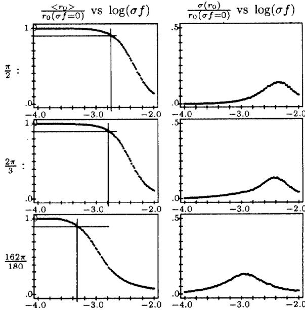
Figure 4: Mean and standard deviation of the shunt impedances of single periodic chains in  $\pi/2, 2\pi/3, 162\pi/180$ -mode vs. standard deviation of the resonance frequencies
