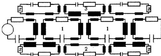
Figure 3: Triple periodic chain with 4 cells, termination impedances and voltage source
