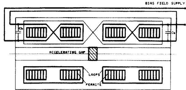
Fig.5 U-70 cavity with loops
