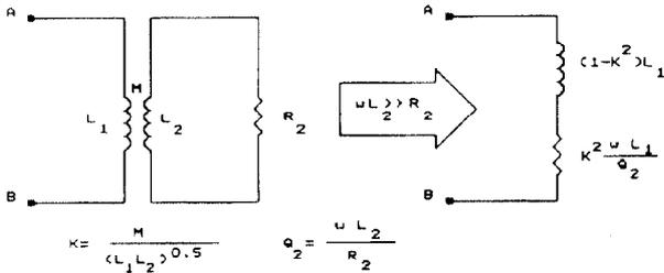
Fig.4 System with an induction coupling principle
