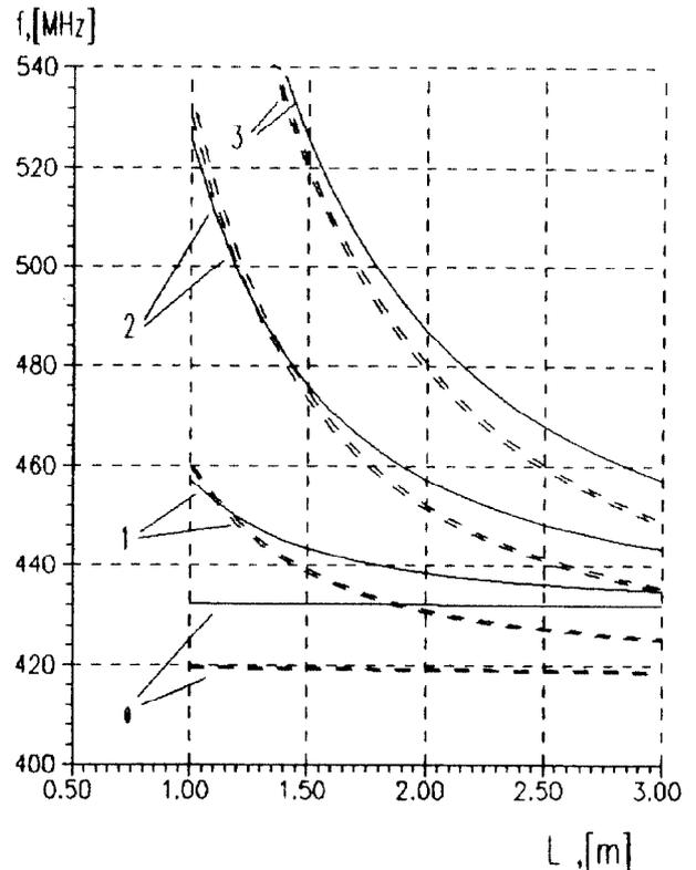
Figure 2. Frequencies of modes as functions of length of resonator.
