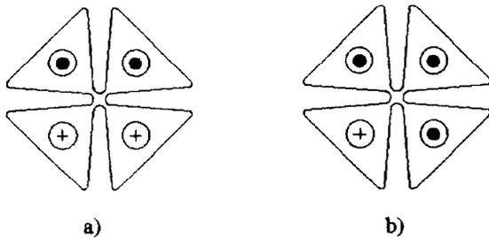
Figure 3.  $H_z$  component of dipole mode.
