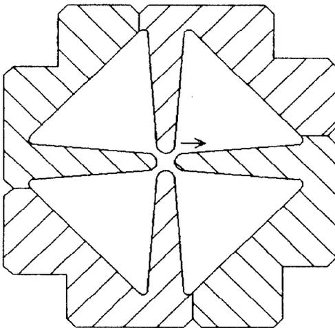
Figure 1. H-resonator cross-section.
