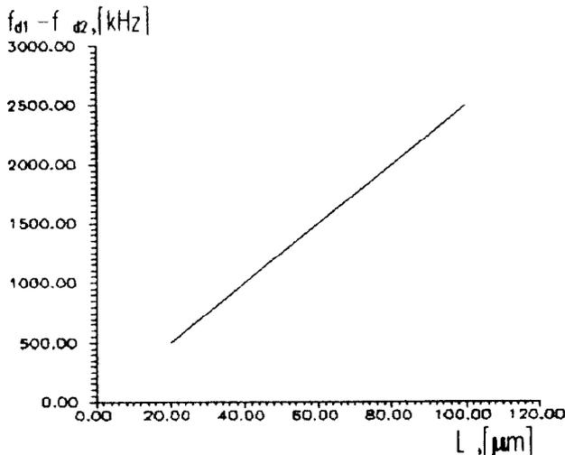
Figure 4. Frequency separation of dipole modes.
