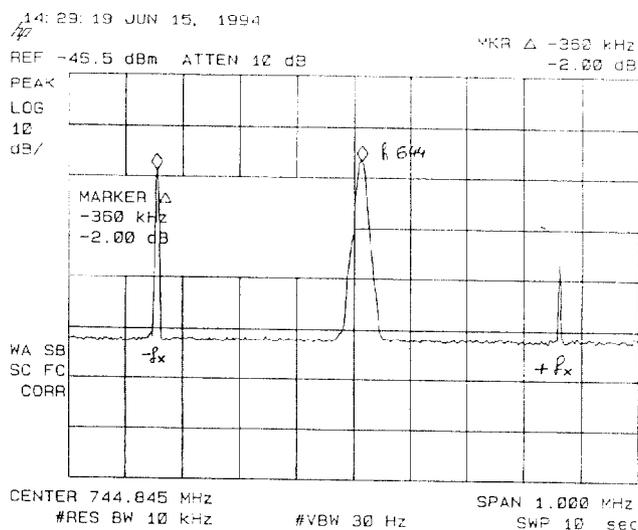
Figure 6. Lower betatron sideband of the harmonic 644, excited when  $T_{ref}$  S2 is above 59.0 °C ( $f_x = 360$  KHz).
