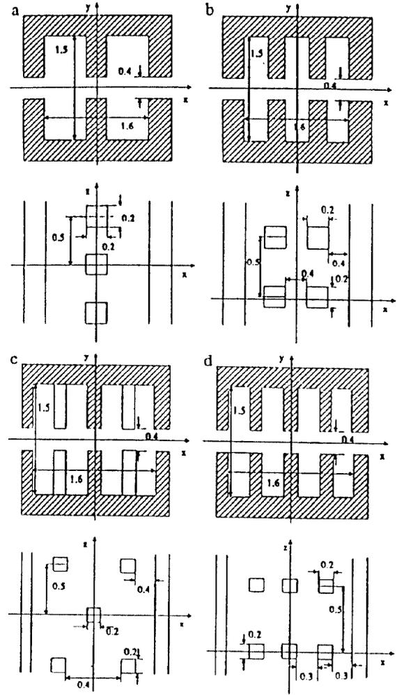
Figure 1. Cross sections and top views of four different RF-structures.
