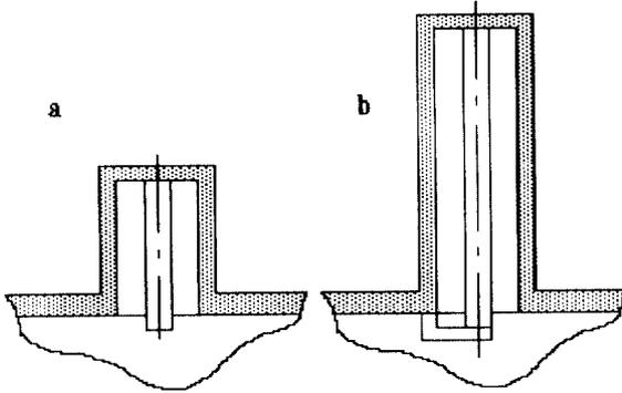
Figure 1. The coaxial absorbing resonator, coupling with accelerating system cavity by means of capacitive (a) or loop (b) coupler.
