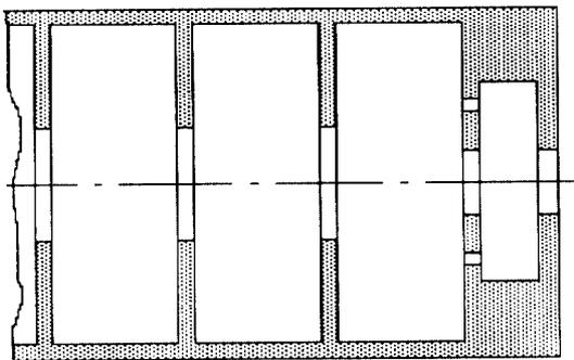
Figure 2. The cylindrical absorbing resonator, coupling with accelerating system cavity by means of the holes in the common wall.
