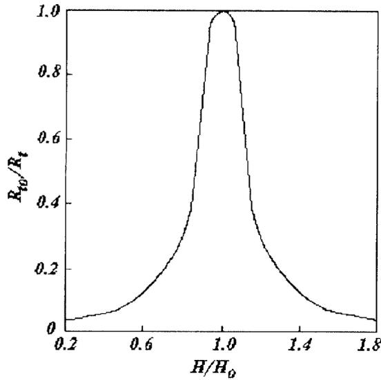
Figure 3. The dependence of transverse shunt impedance  $R_T$  as function of magnetic field  $H$ .
