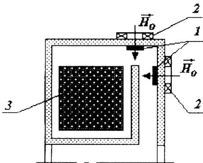
Figure 4. The using of ferromagnetic method in the induction accelerator. 1 - ferrite plate, 2- winding of magnetic system, 3 - core of inductor.
