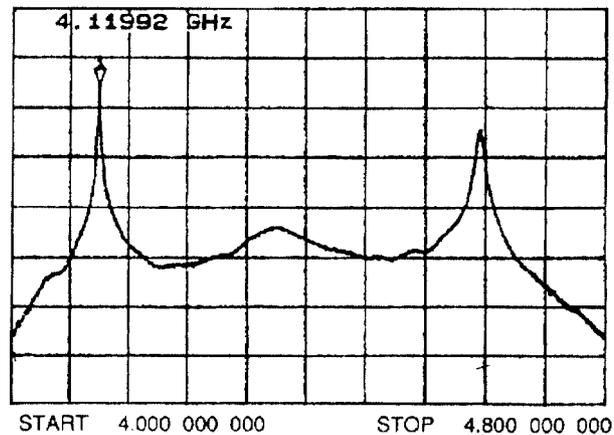
Fig. 3 Mode spectrum of the damped 3-cell cavity. Modes from left to right:  $HEM_{11}-\pi/3$  and  $HEM_{11}-0$  mode. The  $2\pi/3$ -mode has disappeared. Again the third mode belongs to a different passband. (10dB/div. scale).
