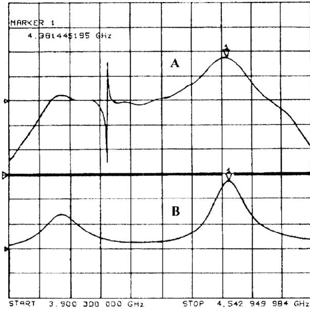
Fig. 4 (A) mode spectrum of the 3-cell structure, coupling through damper waveguide. From left to right:  $HEM_{11}-2\pi/3$ ,  $HEM_{11}-\pi/3$ , and  $HEM_{11}-0$  mode. (5dB/div.). (B)  $|\Delta\Gamma|$  vs frequency. Left:  $HEM_{11}-2\pi/3$ , right:  $HEM_{11}-0$  mode. No coupling to  $HEM_{11}-\pi/3$  mode observed. (5mU/div.).
