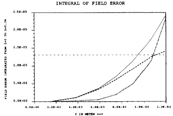
Figure 7. The scaled non-linear field errors at 10 mm.
