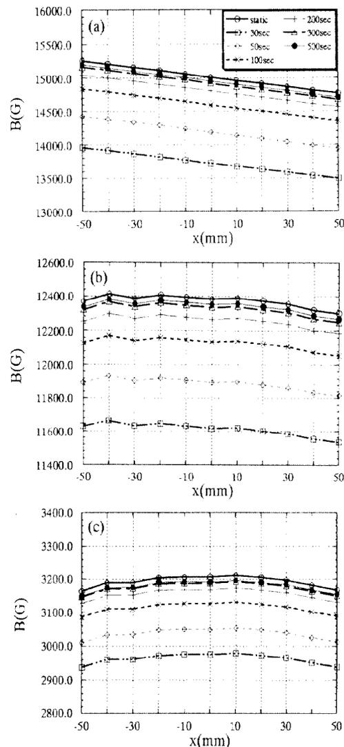
Figure 3 Magnetic field at cross section, (a) 15 deg. from magnet's edge, (b) 1 deg. from magnet's edge, (c) outside of magnet.
