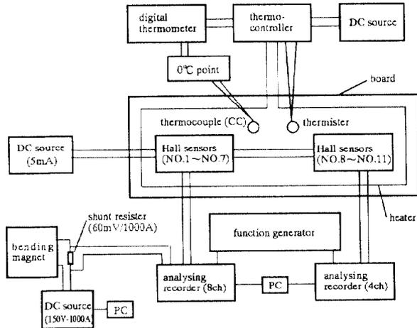
Figure 2 Block diagram of measurement system
