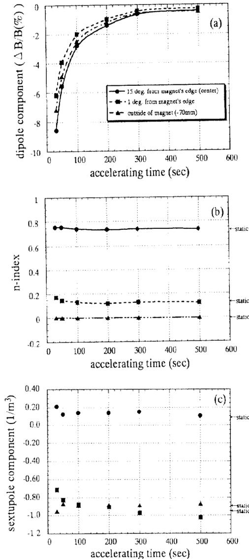
Figure 4 Each component of the magnetic field, (a) the dipole component, (b) the n-index, (c) the sextupole component.
