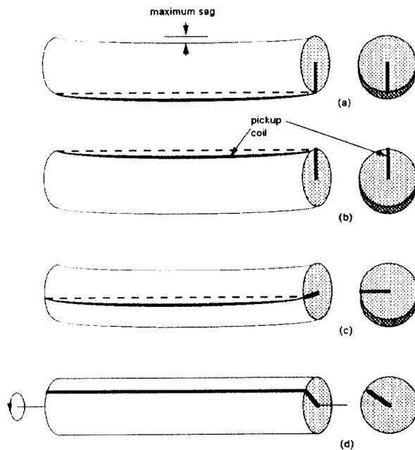
Figure 4. The sag of rotating cylinder due to gravitation. The dashed lines are the positions of the pickup coil after a period of rotation or without sag.
