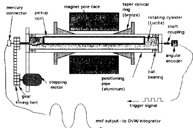
Figure 1. The layout of the rotating coil assembly.
