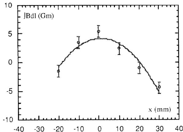
Figure 4. Integrated sextupole term in the wiggler field.
