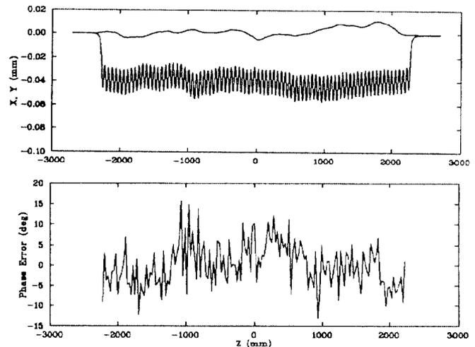
Figure 3. Calculated trajectory and radiation phase in the complete U5.6 undulator at minimum gap.
