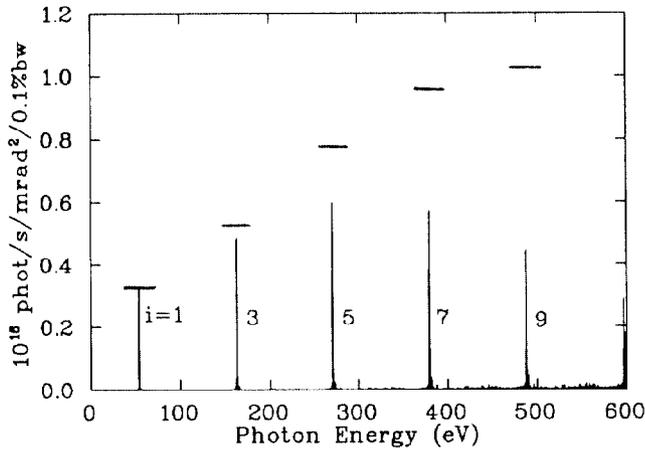
Figure 4. Calculated on-axis spectrum for the complete U5.6 device at minimum gap. The intensities of an ideal undulator are as indicated.
