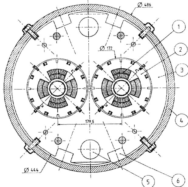
Figure 1. Cross-section of the quadrupole
