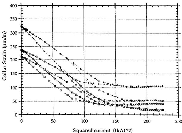
Figure 4. Change in coil prestress during powering to nominal current.
