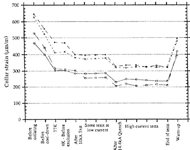
Figure 3. Change in coil prestress during magnet assembly, cool-down, excitation and warm-up.
