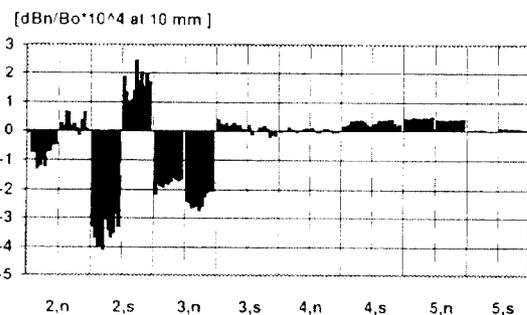
Fig. 5 Relative field errors for 11 adjacent 0.75 m long integrals in the straight part of both apertures at 8.65 T. The harmonics go from normal quadrupole (2,n) to skew decapole (5,s)
