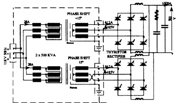
Figure 1 - Electrical Circuit of 750kW Power Converter
