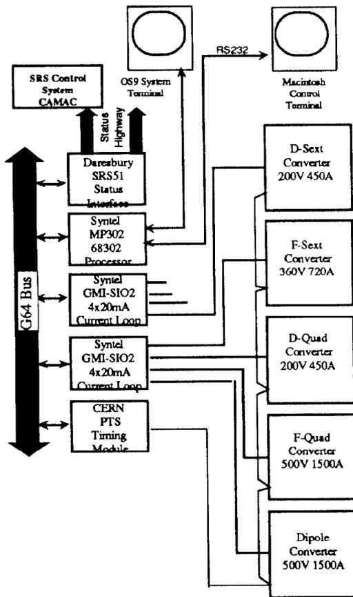
Figure 2. Block Diagram of Power Converter Control System
