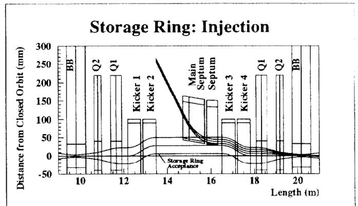
Figure 6: Top view of the injection section of the storage ring. Sketched are the  $3\sigma_x$  - envelopes of the injected beam, the maximum closed orbit distortion and the acceptance.
