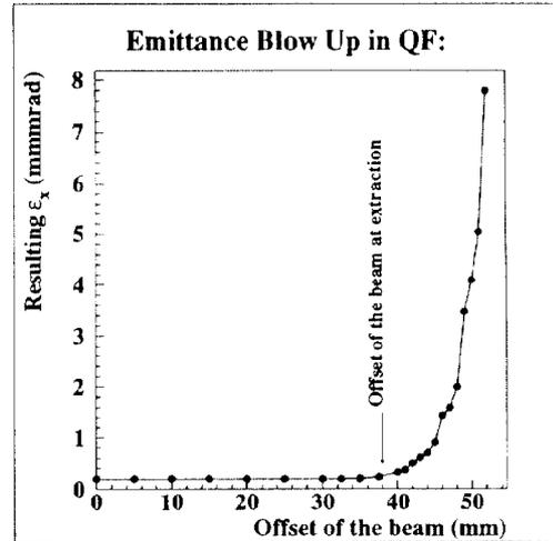
Figure 5: Emittance growth as a function of the beam's offset when passing the last quadrupole QF at extraction.
