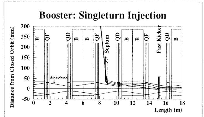
Figure 1: Injection region for the singleturn injection into the booster
