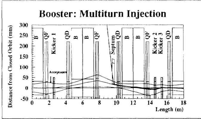
Figure 3: Top view of the injection region for the multiturn injection into the booster. The  $3\sigma_x$  - envelope, the maximum closed orbit distortion and the booster acceptance are illustrated.
