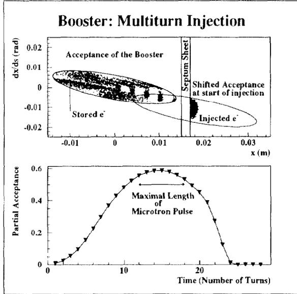
Figure 2: Phase space diagram of multiturn injection and partial acceptance as a function of time for a septum thickness of 2 mm and a horizontal tune of the Booster of  $Q_x = 4.4$ .
