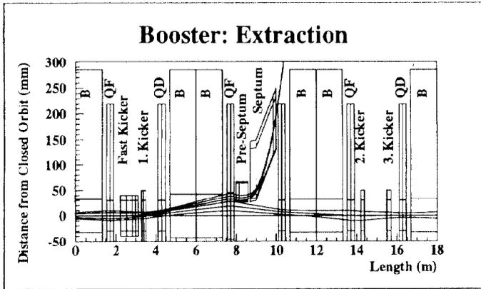
Figure 4: Top view of the extraction region of the booster. The  $3\sigma_x$  - envelopes for the distorted and extracted beam are shown.
