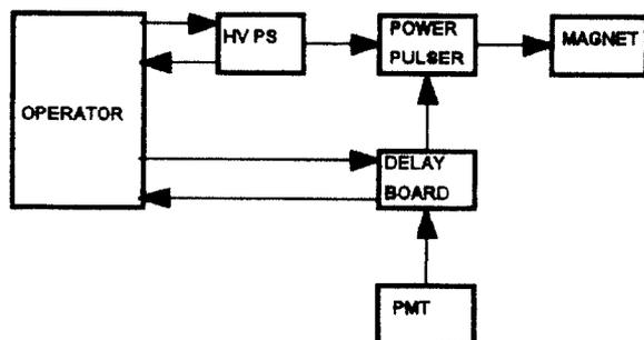
Fig. 1 - Typical pulsed magnet system block diagram
