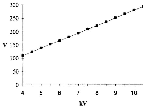
Fig. 7 - Signal from Kicker CT vs. HV
