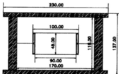
Fig. 2 Kicker Magnet cross section
