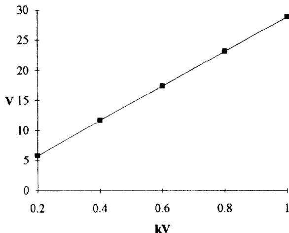
Fig. 8 - Signal from Septum CT vs. HV
