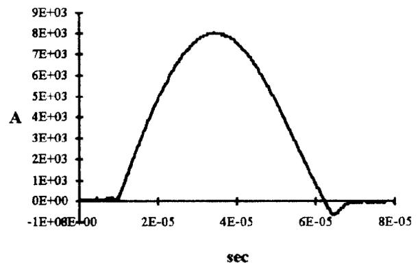
Fig. 6 - 8 kA Septum current pulse
