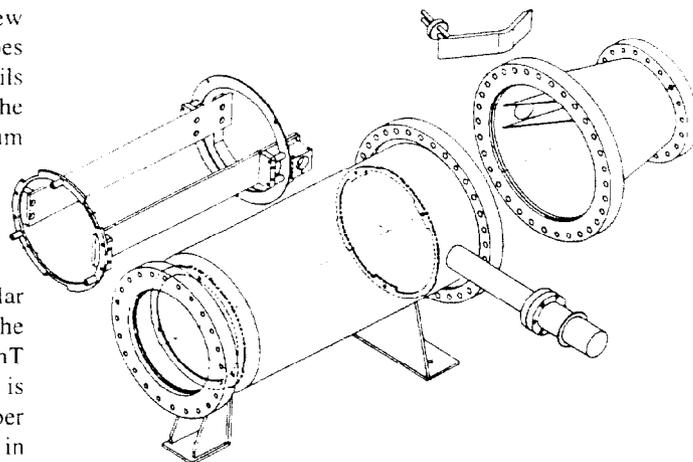
Figure 2. Exploded view of Kicker and its Vacuum vessel.
