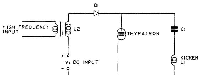
Figure 3. Simplified circuit diagram of pulsed power supply.
