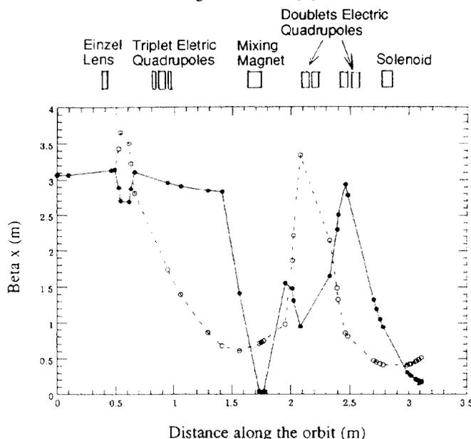
Fig. 1  $\beta$ -functions of the existing transport line from the ion source to the RFQ.
