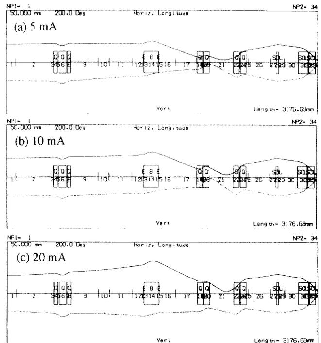
Fig. 5 Beam envelopes for various currents at the modified transport line.
