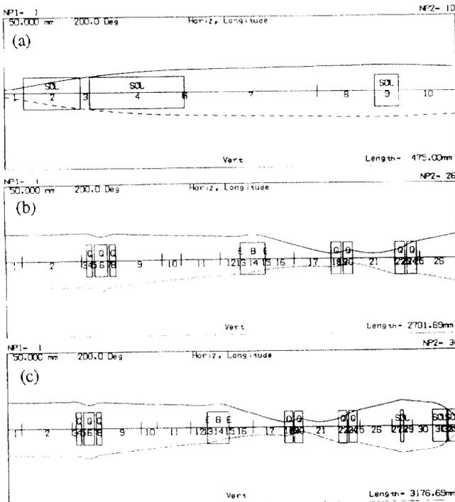
Fig. 4. Design procedure of transverse phase space matching at the new beam optics for 0 mA.
