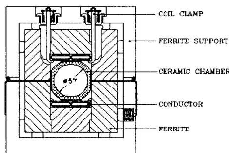
Figure 1: Cross-section of the kicker magnet
