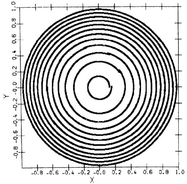
Figure 1. Bunched beam scanning of a target.
