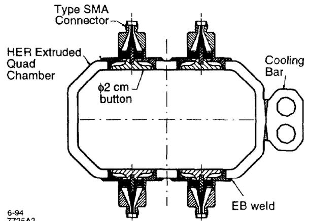
Figure 5 Cross section of quadrupole chamber showing BPM feedthroughs.
