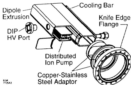
Figure 2 Isometric view of HER dipole vacuum chamber
