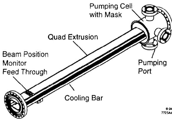
Figure 4 Isometric view of quadrupole vacuum chamber.
