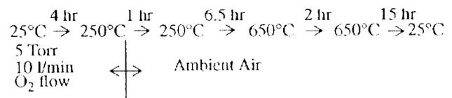
Heraeus calls for a different firing cycle with a peak temperature of 800 °C for 20 minutes. However, before coating, our tubes already have a Kovar flange brazed to them. The brazing joint melts at  $\approx 680$  °C thus we cannot heat the tubes to 800 °C. Nevertheless, we have found that many of the Heraeus pastes fully sinter at lower temperatures provided they are in the oven for a long enough period.
