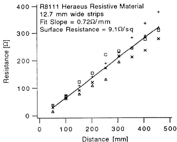
Figure 2: Measured resistance of four individual 12.7-mm-wide R8111 strips on a painted and fired ceramic substrate.
