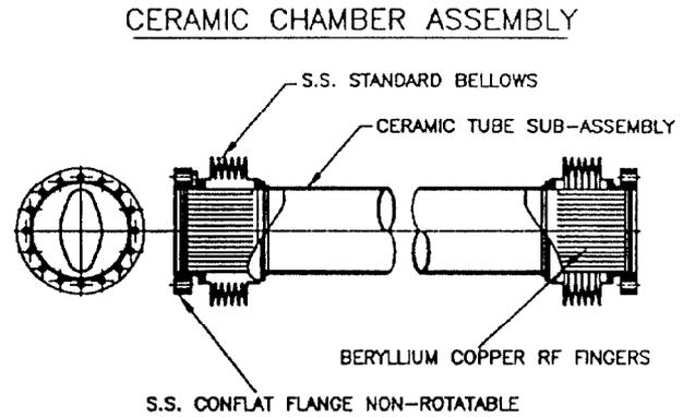
Figure 1: The SR Ceramic Tube Assembly
