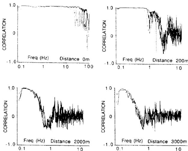
Fig.3 Correlation spectra for vertical vibrations
