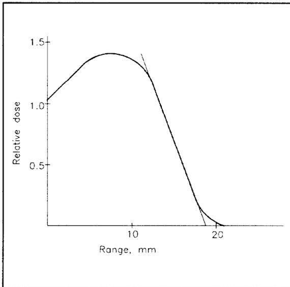
Fig. 2. Electron absorption curve measured with the use of aluminum wedge with dimensions of 100 x 60 x 30 mm and PVC dosimetric foil, at pulse duration  $5\mu\text{s}$ , PRR = 300 Hz and pulse beam current 400 mA.
