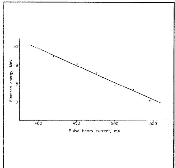
Fig. 3. Beam loading curve, measured at average magnetron current 0.75A, pulse duration  $5\mu\text{s}$  and pulse repetition ratio 300 Hz.
