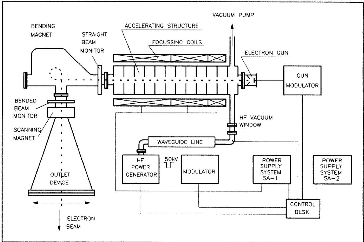
Fig. 1. Electronica 10-10 accelerator's block diagram.
