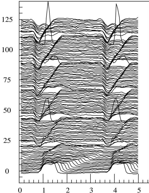
Figure 3: Mountain range display of beam current for 6 transfers. There are  $6.0\text{ms} = 2048$  turns between traces and the horizontal axis is in  $\mu\text{s}$ .
