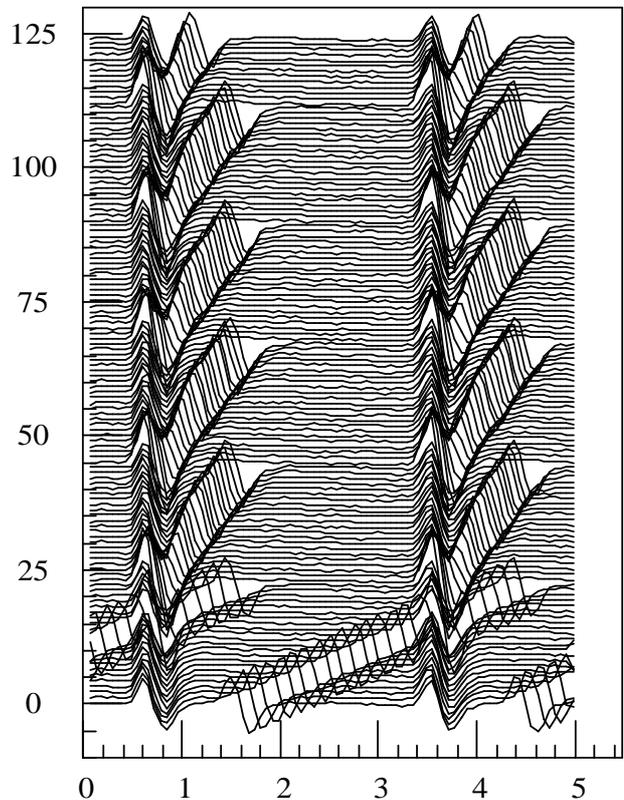
Figure 2: Mountain range display of the sum of the rf voltage from the two barrier cavities for 6 transfers. There are  $6.0 \text{ ms} = 2048$  turns between traces and the horizontal axis is in  $\mu\text{s}$ , ( $2.9 \mu\text{s}$  per turn).
