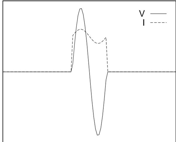
Figure 1: Barrier cavity voltage and current for one turn.
