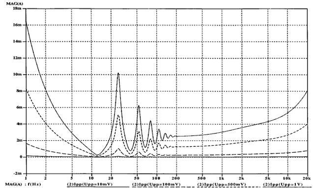
Figure 5: Total current ripple as function of frequency.
