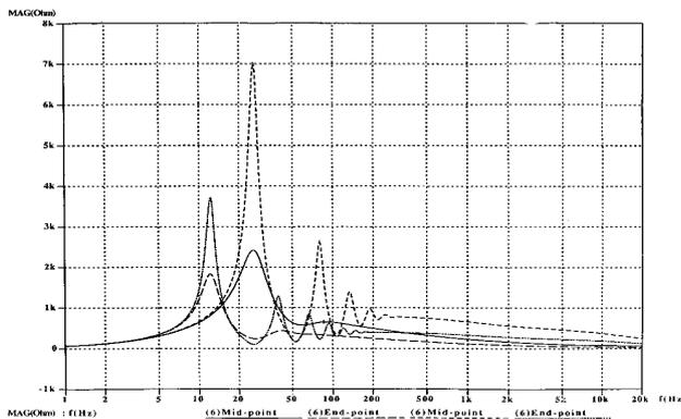
Figure 4: Total load impedance w.r.t. frequency.
