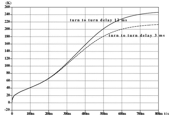
Figure 3: MCBX : Hot spot temperature versus time for turn-to-turn delays of 3 ms and 12 ms
