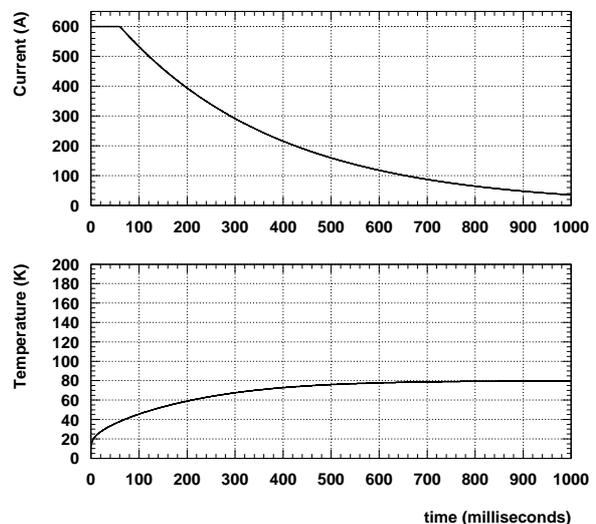
Figure 4: MCBX : Current and temperature versus time for magnet with external resistor of  $0.5 \Omega$ ,  $RRR = 120$
