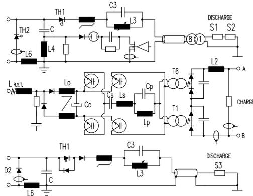
Fig.3: Electrical diagram of power converters
