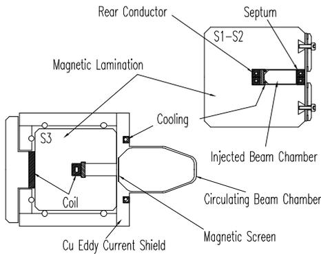
Fig.2: Cross-section of S1-S2 and S3 magnets
