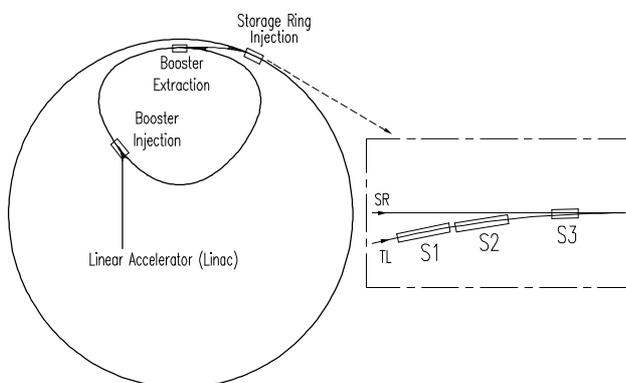
Fig.1: ESRF complex and SR injection layout.
