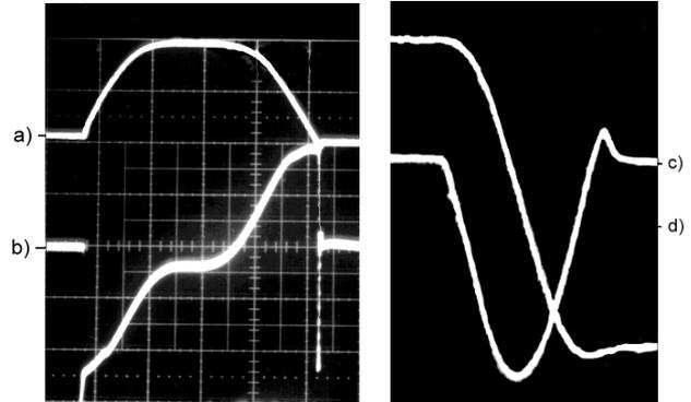
Fig 4: Wave shapes recorded during tests: S1-S2 at 9 kA: a) Magnet current (5 kA/d-0.5 ms/d); b) Transformer primary voltage (0.8 kV/d). S3 at 8 kA: c) Magnet current (2 kA/d-20  $\mu\text{s}/\text{d}$ ); d) Capacitor voltage (0.5 kV/d)
