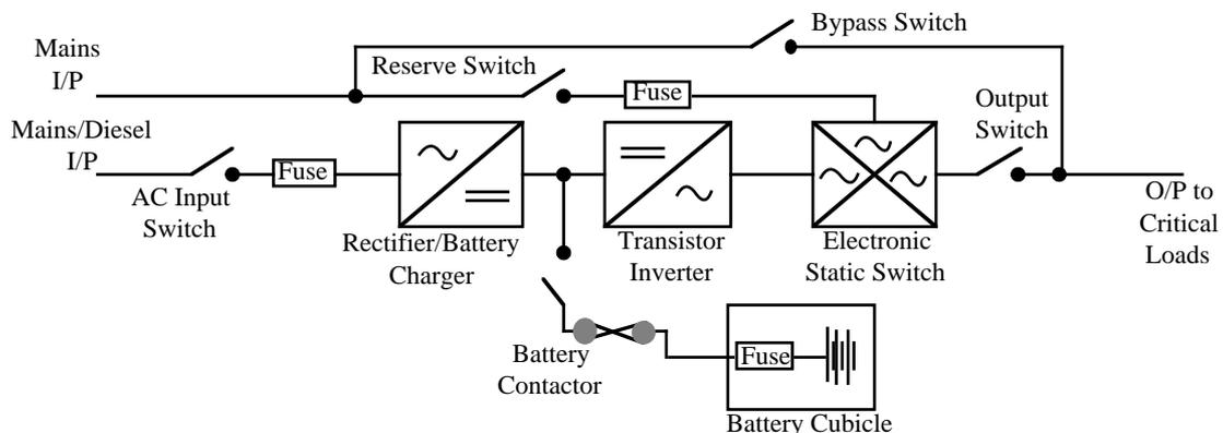
Figure 2 : UPS Circuit Diagram
