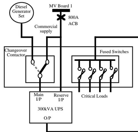
Figure 1: UPS Connection Diagram
