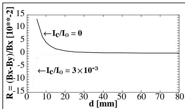
Figure 6: Field difference ratio  $R$ , in percent, as a function of distance from origin (coordinates as shown in Fig. 5).
