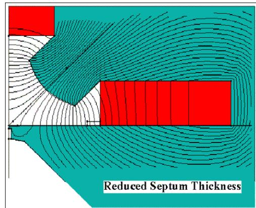
Figure 2: MSQ same as Fig. 1 but with additional 2 $\times$ 8 mm cut leaving 2 mm thick septum.
