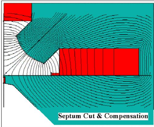
Figure 4: MSQ same as Fig. 2 but with correction coil in 2×8 mm cut. Return coil is mounted on mirror plate.
