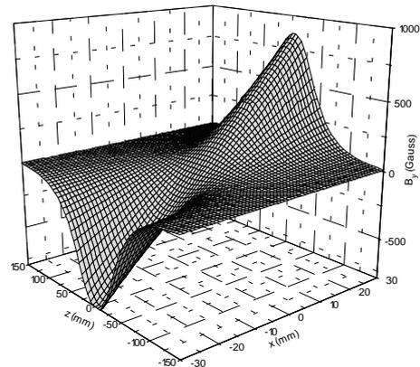
Figure 5 Measured flux density of the PMQ using a Hall probe
