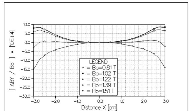
Fig. 3: The homogeneity of the magnetic field
