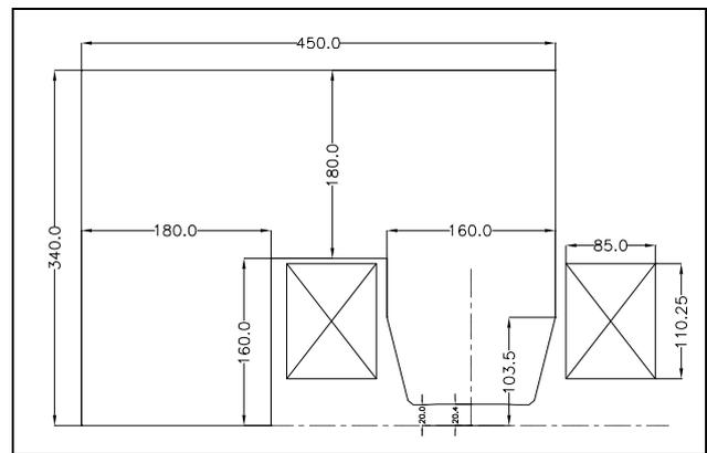
Fig.1: Cross section of the ANKA bending magnet.
