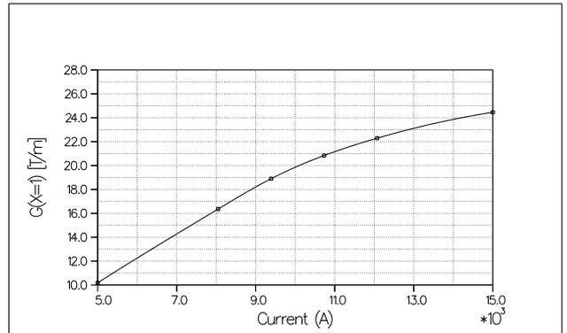
Fig. 7: Excitation curve for the ANKA-quadrupole.
