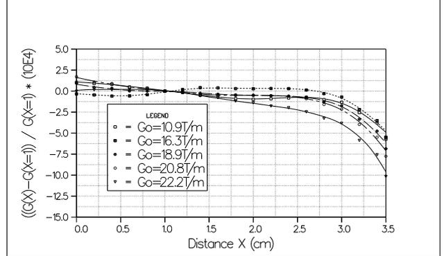
Fig. 6: The homogeneity of the gradient within the quadrupole
