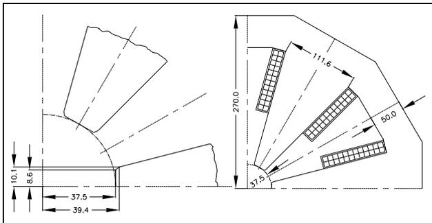
Fig. 8: Lamination and pole profile for the ANKA sextupole.
