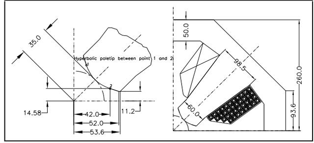
Fig. 5: Lamination and pole profile for the ANKA quadrupole.
