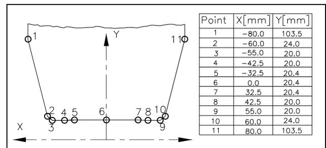
Fig.2: The pole profile of the bending magnet.
