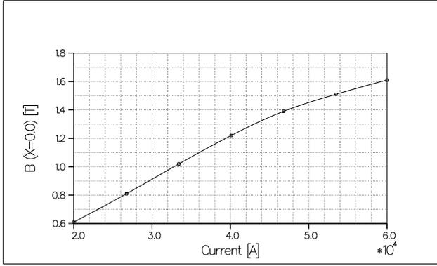
Fig. 4: The excitation curve of the ANKA bending magnet.
