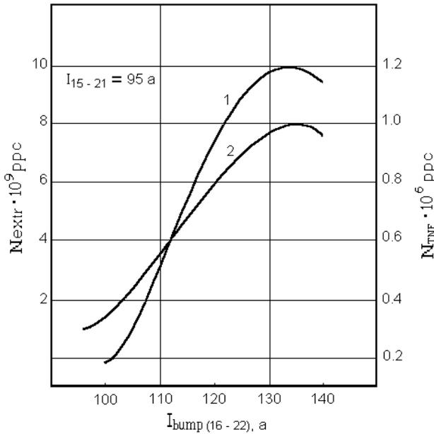
Figure 2: Dependencies of intensity of extracted protons (curve 1) and K-mesons after the target of the experimental setup ( curve 2) versus the current of a bump formed by magnetic blocks 16, 22 of the accelerator.
