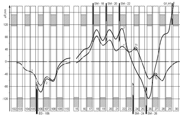
Figure 1: The scheme of a proton beam extraction. ED-106, SM-18, 20, 22, 26 are the electrostatic and magnetic deflectors; Q<sub>1</sub>, H<sub>1</sub> are the first elements of the beam transport system; SM-24 is the septum--magnet of the fast ejection system; T<sub>1</sub>, T<sub>2</sub> are the internal targets of channels 2(14) and 4, respectively.
