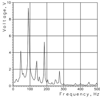
Figure 2: Voltage ripple at power supply
