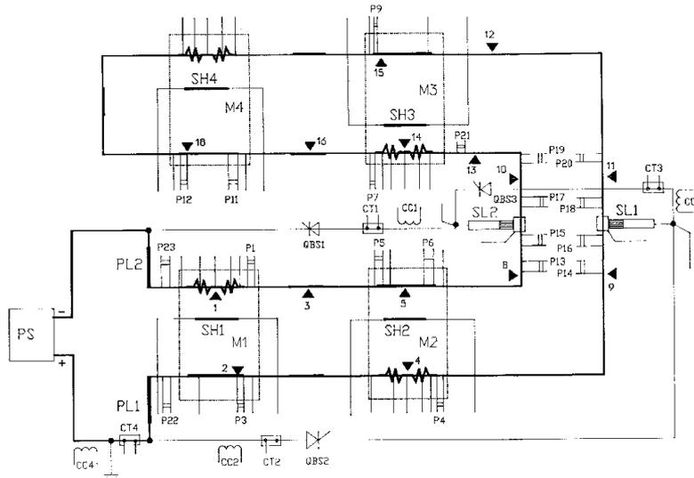
Figure 2: Electrical diagram of 4 magnet string: M1–M4 — SC dipole magnets, PS — power supply, PL — power lead, SL — safety leads, QBS — quench bypass switch, CT — current transducer, SH — strip heaters, ▽ — spot heaters, P1–P23 — potential taps.
