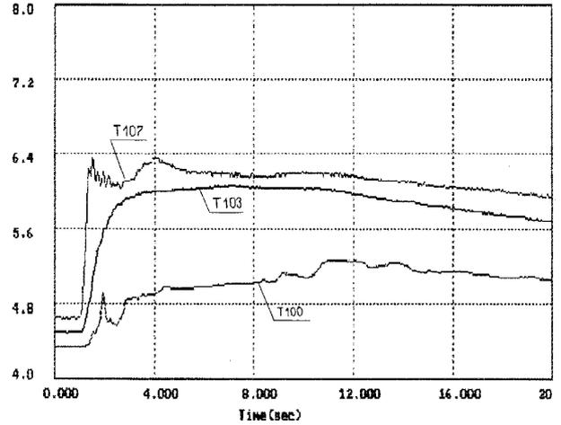
Figure 4: Time dependence of temperature during quench induced by  $\nabla 10$ : T100 — inlet helium temperature, T103, T107 — temperature of QS near SC cable soldering.
