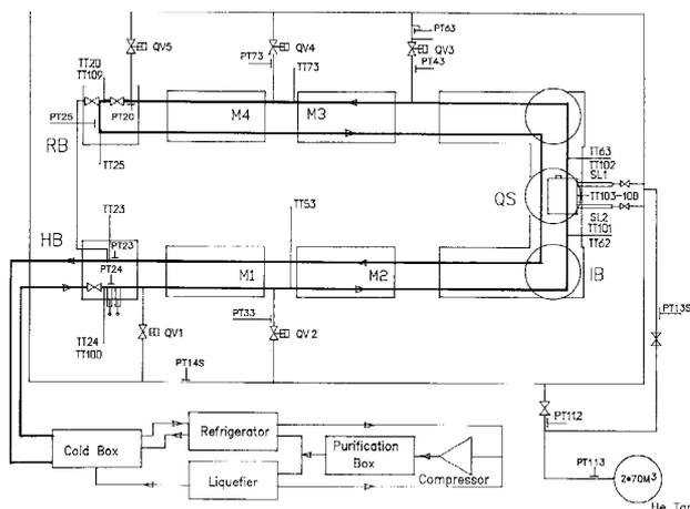
Figure 1: Cryogenic diagram of 4 magnet string: HB — head box, IB — intermediate box, RB — return box, QS — quench stopper, QV — quench valves, SL — safety leads, TT — temperature transducer, PT — pressure transducer.
