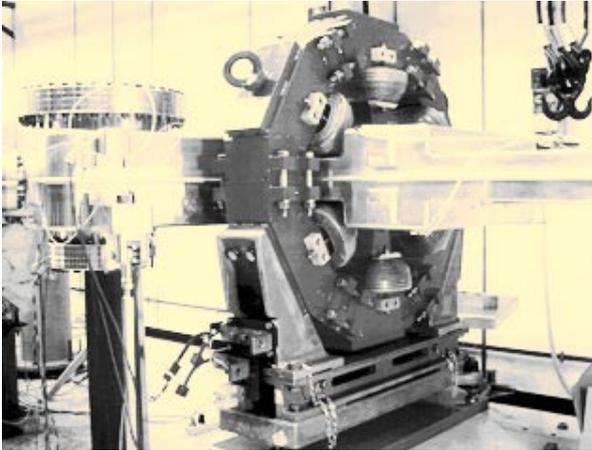
Figure 7 - The sextupole prototype assembled on the arc vacuum chamber.
