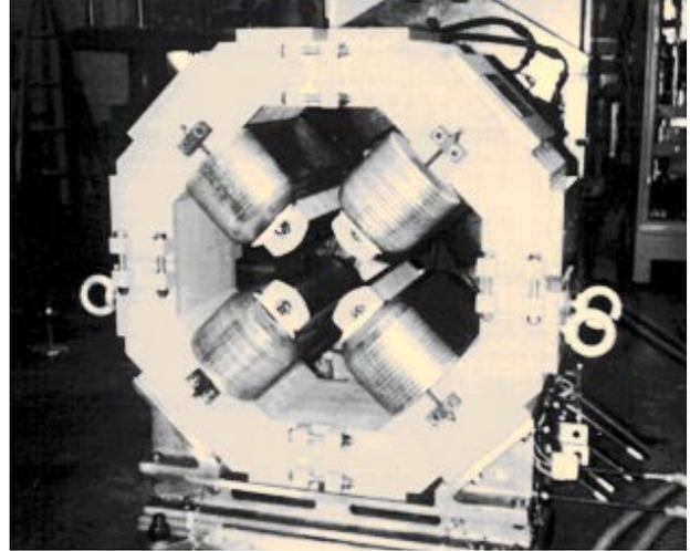
Figure 4 - Large Quadrupole Prototype.
