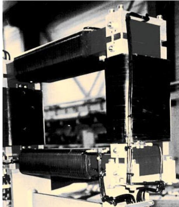
Figure 9 - The HV Rectangular Corrector Magnet
