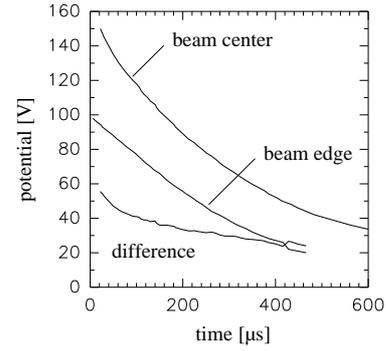
Figure 2: The potential of the beam center and the beam edge of an ion beam ( $\text{He}^+$ , 10 keV, 3 mA) as function of time ( $5 \cdot 10^{-5}$  hPa He RG pressure).
