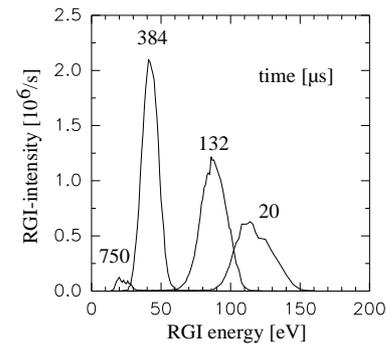
Figure 4: Some dynamic RGI energy spectra of an ion beam ( $\text{He}^+$ , 10 keV, 3 mA) at certain times ( $5 \cdot 10^{-5}$  hPa He RG pressure).
