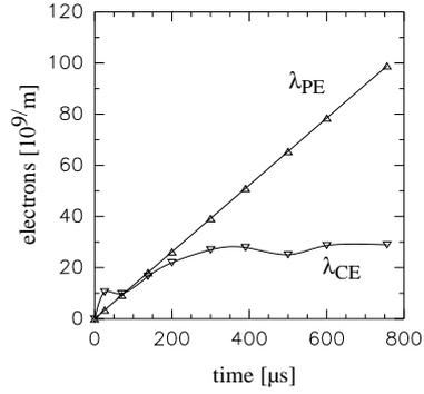
Figure 7: Electron line density of the produced ( $\lambda_{\text{PE}}$ ) and the captured ( $\lambda_{\text{CE}}$ ) electrons as a function of the time after the start of the SCC ( $\text{He}^+$ , 10 keV, 3 mA,  $5 \cdot 10^{-5}$  hPa He RG pressure).
