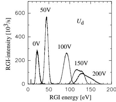
Figure 3: Some static RGI energy spectra of a partially compensated (electrode biased to  $U_d$  to decompensate the beam) ion beam ( $\text{He}^+$ , 10 keV, 3 mA).
