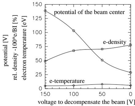
Figure 6: Relative electron density and temperature and the potential of the beam in the static case as a function of the decompensation voltage obtained by self-consistent calculations ( $\text{He}^+$ , 10 keV, 3 mA,  $5 \cdot 10^{-5}$  hPa He RG pressure).
