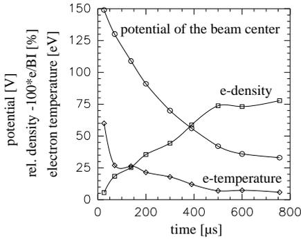
Figure 5: Relative electron density and temperature and the potential of the beam in the dynamic case as a function of the rise time obtained by self-consistent calculations ( $\text{He}^+$ , 10 keV, 3 mA,  $5 \cdot 10^{-5}$  hPa He RG pressure).
