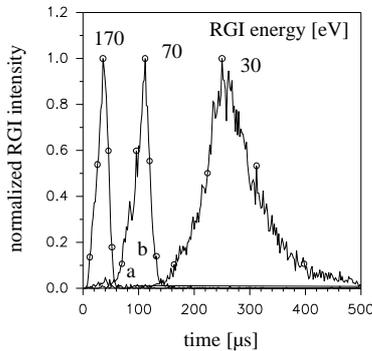
Figure 1: Some typical dynamic RGI intensities at certain RGI energies of an ion beam ( $\text{He}^+$ , 10 keV, 4.8 mA) as function of time after the start of the compensation ( $4 \cdot 10^{-5}$  hPa He RG pressure).
