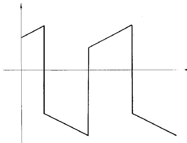
Figure 1: Ideal voltage waveform for a linear scanning magnet
