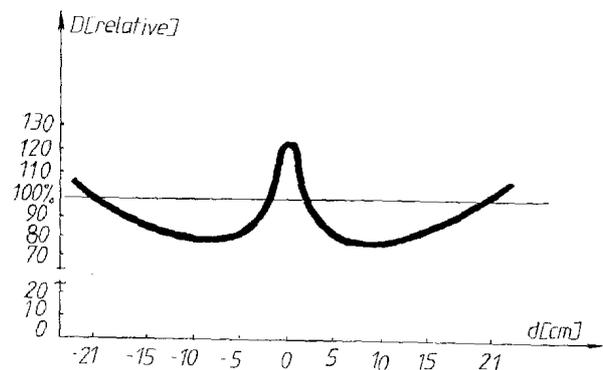
(b) scanning magnet coils fed with a 50 Hz sinusoidal waveform and with a third-harmonic component (6% from the 50 Hz fundamental amplitude).
