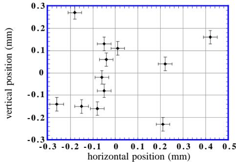
Figure 1: Horizontal and vertical position of the 12 quadrupoles centres of the experimental line. Goal: 0.3 mm RMS. Achieved: 0.2 mm RMS.
