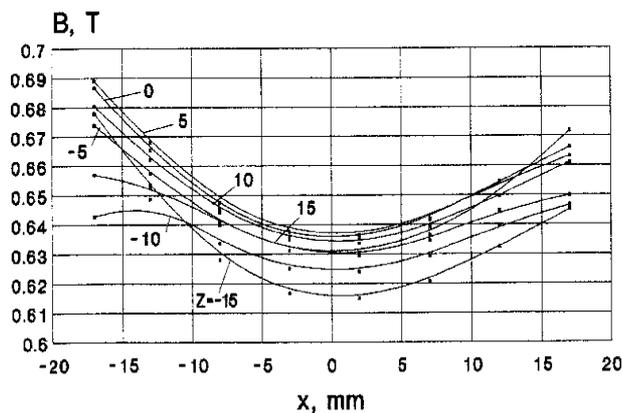
Figure 3. Field distribution in the pole plane of the dipole for 7 cross-sections; points - measured data, curves - smooth approximation lines.
