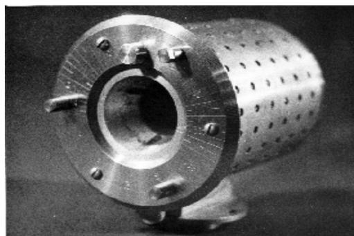
Figure 1. The PM split-pole dipole with variable field.
