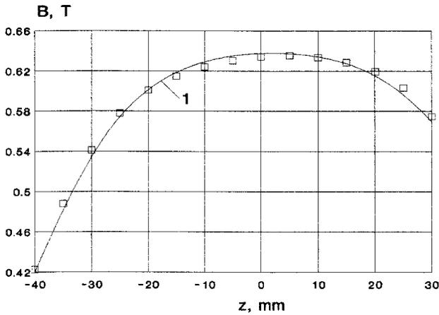
Figure 2. Dipole field  $z$ -dependence near its geometrical centre; measured data - (points), calculated curve - (1).
