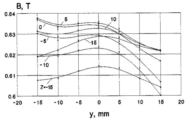
Figure 4. Field distribution in the median plane of the dipole for 7 cross-sections; points - measured data, curves - smooth approximation lines.
