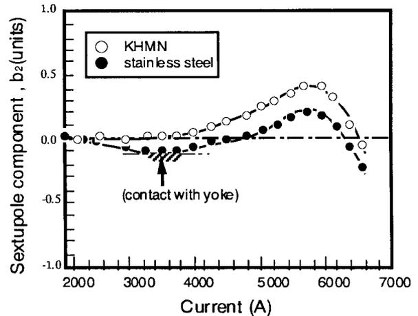
Fig. 5 Change in sextupole error component with current in dipole small magnets with KHMN and stainless steel collars (SSCL)
