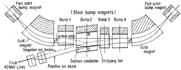
Figure: 1 Injection system for positive-negative ions
