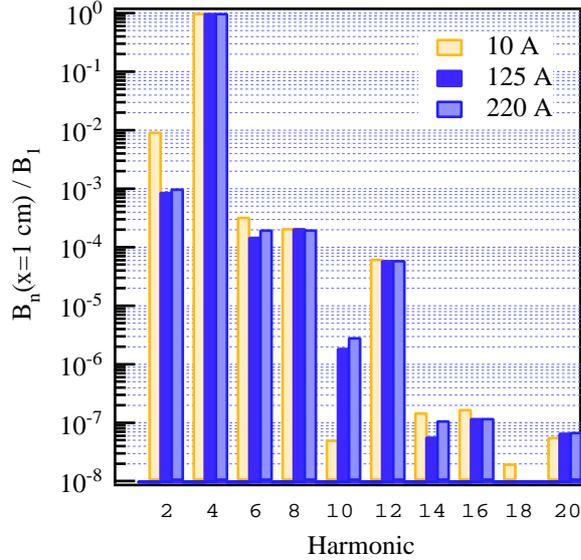
Figure 6: Harmonic analysis in the geometric center., Multipole field components normalized to the quadrupole component at 1 cm from center. Values are within specified tolerances.
