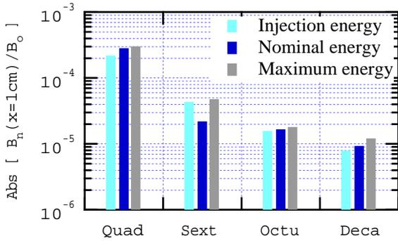
Figure 3: Dipole multipole field components. Except for the quadrupole term, which is now incorporated in linear optics calculations, the results show that the dipoles are adequate.
