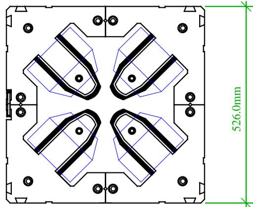
Figure 4: Quadrupole cross section. Length:  $250.4 \pm 0.5$  mm. Turns per coil: 37. Power @225A: 1700 W. Gradient @225A: 18 T/m, 1.5% saturation.
