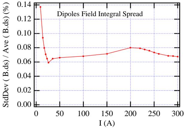
Figure 2: R.m.s. spread in measured excitation curves for the 12 dipoles. The specified tolerance for excitation error is 0.1% r.m.s. Note that the spread at injection current (19 A) is already within specified value.
