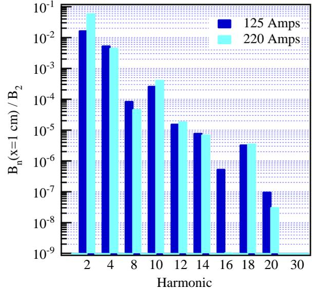
Figure 8: Sextupole multipole field components normalized to the main component at 1 cm from the magnet center.
