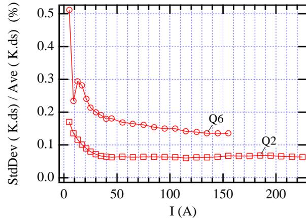
Figure 5: R.m.s. spread in measured excitation curves for the 2 and 6 quadrupole families. The specified tolerance for excitation error is 0.2%.
