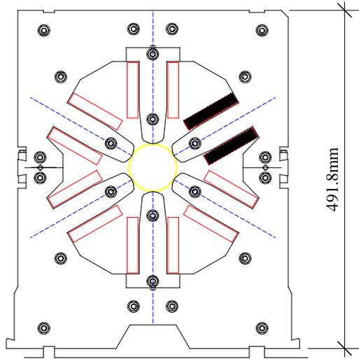
Figure 7: Sextupole cross section. Core length:  $99.1 \pm 0.3$  mm. Turns per coil: 20. Power @225 A: 1400 W. Gradient @150 A: 635 Tesla/m<sup>2</sup>, 1% saturation. Gradient @200 A: 770 Tesla/m<sup>2</sup>, 15% saturation. Effective length: 120 mm.
