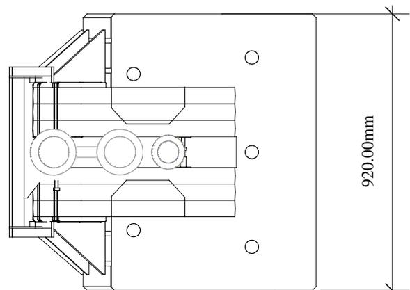
Figure 1: Dipole cross section. Length: 1.442 m. Bend. radius: 2.735 m. Gap: 58 mm. Field (@300A): 1.65 T.
