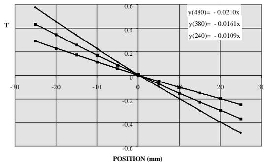
When measuring the lattice multipole magnets a back leg current is added to adjust the dipole component to a minimum. With this correction it was found that the excitation dependence of the integrated sextupole is closely following that of the integrated gradient.
